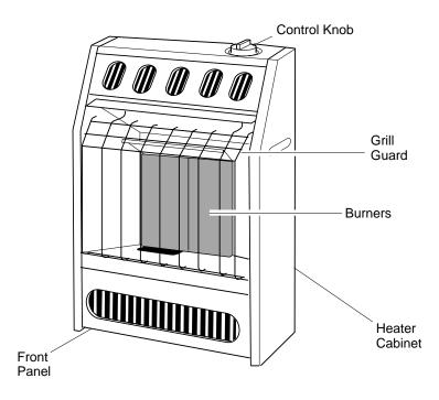
Figure 1 - Vent-Free Propane/LP Gas Heater
